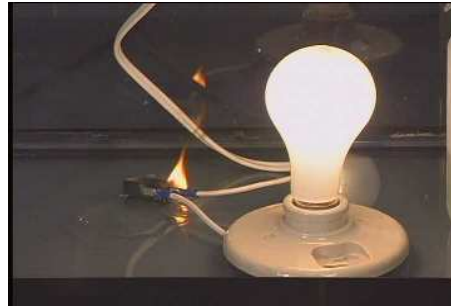
Fig. 5, Example of ignition of gasses from switch plastic by arc tracking across the charred plastic surface of the switch due to the presence of conductive liquid on the switch.
